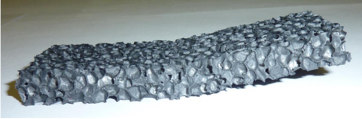
Figure 1: Closed-cell aluminum foam specimen after laser forming
