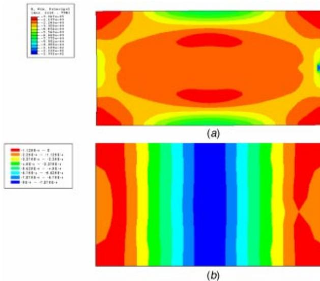
Fig. 5 (a) Minimal principal in-plane strain, and (b) minimal principal bending strain for the saddle shape (dimension: 140\*80\*0.89 mm<sup>3</sup>)
