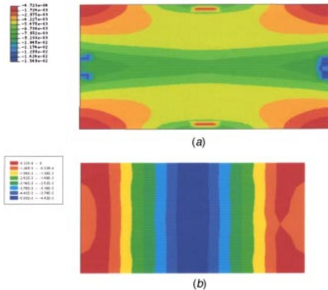
**Fig. 13 (a) Minimal principal in-plane strain, and (b) minimal principal bending strain for the saddle shape of thicker plate (dimension: 140\*80\*5 mm<sup>3</sup>)**
