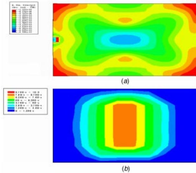
Fig. 4 (a) Minimal principal in-plane strain, and (b) minimal principal bending strain for the pillow shape (dimension: 140\*80\*0.89 mm<sup>3</sup>)
