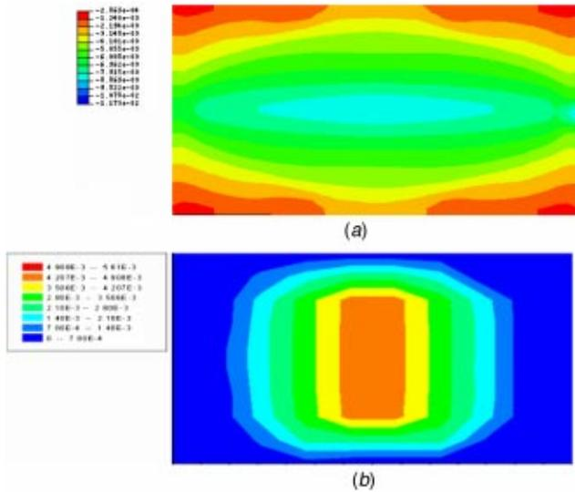
**Fig. 12 (a) Minimal principal in-plane strain, and (b) minimal principal bending strain for the pillow shape of thicker plate (dimension: 140\*80\*5 mm<sup>3</sup>)**
