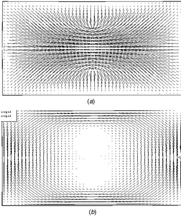
**Fig. 6** Vector plots of minimal principal in-plane strain for (a) pillow shape, and (b) saddle shape (the orientation of segments indicates strain direction and length of segments indicates strain magnitude)
