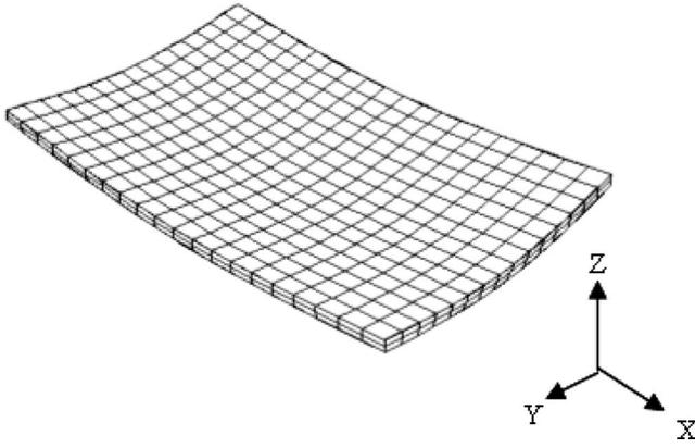
Fig. 2 Desired shape I: pillow (dimension: 140\*80\*0.89 mm<sup>3</sup>, magnification ×5 in thickness for viewing clarity)
