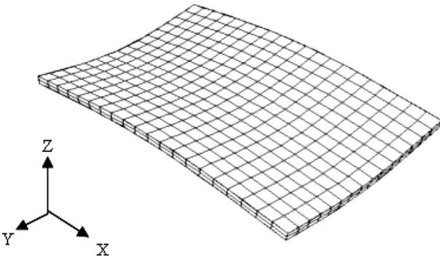
Fig. 3 Desired shape II: saddle (dimension: 140\*80\*0.89 mm<sup>3</sup>, magnification ×5 in thickness for viewing clarity)
