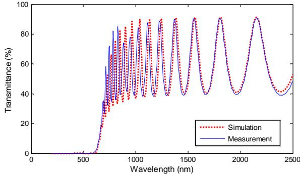
**Figure 4 Comparison of transmittance spectra for both simulation and measurement by spectrophotometry of as-received a-Si:H film on glass substrate, film thickness is 1.6µm**
