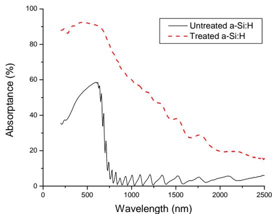
**Figure 8 Comparison of absorptance spectra measurement of as-received and laser treated a-Si:H film by spectrophotometry (fluence of  $0.5\text{J}/\text{cm}^2$ , scan at  $25\text{mm}/\text{s}$ ), showing increase in absorptance over entire spectrum**
