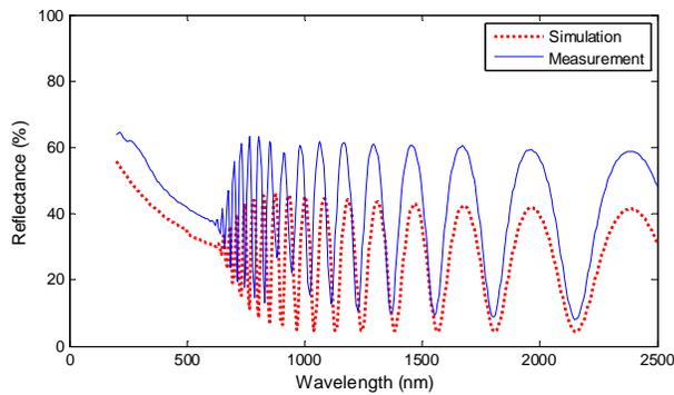
**Figure 5 Comparison of reflectance spectra for both simulation and measurement by spectrophotometry of as-received a-Si:H film on glass substrate, film thickness is 1.6µm**
