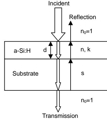
**Figure 3 Schematic of one-dimensional absorption simulation model of as-received a-Si:H film on glass substrate, film thickness  $d=1.6\mu\text{m}$ , real and imaginary parts of refractive index of a-Si:H film are  $n$  and  $k$ ,  $s$  and  $n_0$  are the refractive index of the substrate and air**
