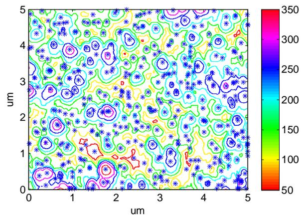
**Figure 13 Schematic of peak identification of extraction data from AFM images of laser irradiated a-Si:H film at different fluence and number of pulses, star means the identified peak point, solid curves indicate the contour spectra, AFM scanning area is  $5\times 5\text{ }\mu\text{m}$ , color bar unit: nm**
