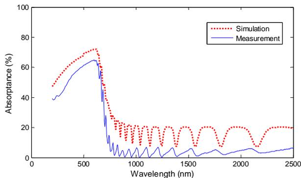
**Figure 6 Comparison of calculated absorptance spectra ( $A=100-T-R$ ) of as-received a-Si:H film on glass substrate based on both transmission and reflection simulation and measurement by spectrophotometry, film thickness is 1.6µm**
