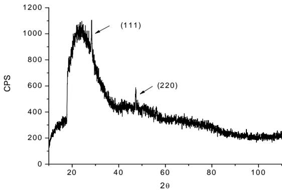
**Figure 10 XRD spectrum of laser treated a-Si:H film at fluence of  $0.5\text{J}/\text{cm}^2$  and scanning speed of  $25\text{ mm/s}$ , an “amorphous peak” around  $2\theta=25^\circ$ , existence of two overall different peaks for (111) and (220) orientation of silicon**
