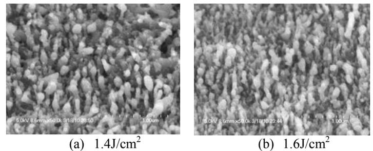
**Figure 12 SEM images of laser irradiation of a-Si:H film for 50 pulses at fluence of (a)  $1.4\text{J}/\text{cm}^2$  (b)  $1.6\text{J}/\text{cm}^2$ , the irradiation spot diameter is  $150\text{ }\mu\text{m}$ , showing similar spikes distributed on the surface**
