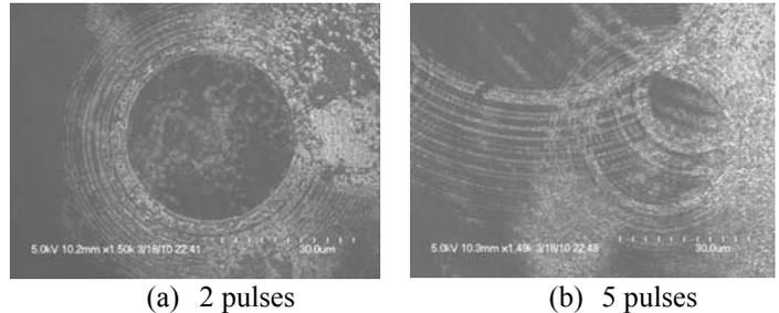
**Figure 11 SEM images near the edge of laser irradiation area on a-Si:H film for (a) 2 pulses (b) 5 pulses at the fluence of  $1.4\text{J}/\text{cm}^2$ , the irradiation spot diameter is  $150\text{ }\mu\text{m}$ , showing superposition of diffraction fringes from separate bubbles**
