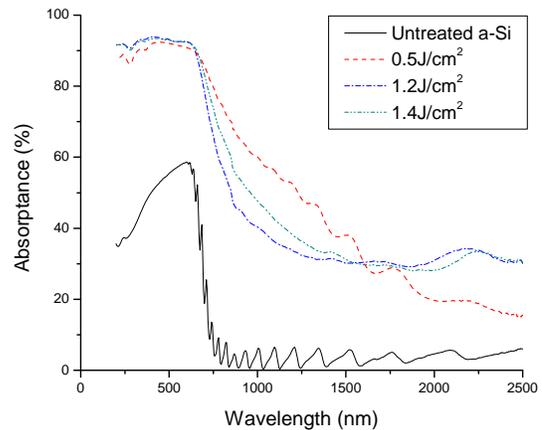
**Figure 16 Comparison of absorptance spectra measured by spectrophotometer of as-received and laser irradiated a-Si:H film at different fluence and pulse overlap ( $0.5\text{J}/\text{cm}^2$  at  $25\text{mm}/\text{s}$ ,  $1.2\text{J}/\text{cm}^2$  at 50 pulses,  $1.4\text{J}/\text{cm}^2$  at 20 pulses), showing enhanced absorptance for all processed samples**
